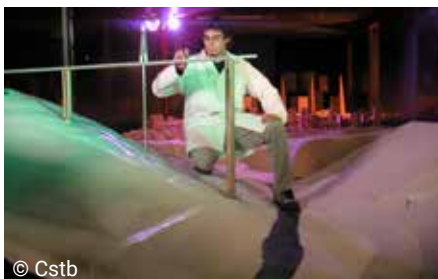
Aeroelastic model of a construction stage
