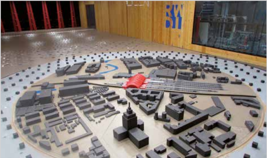
Riga station model in RWDI wind tunnel Lab
