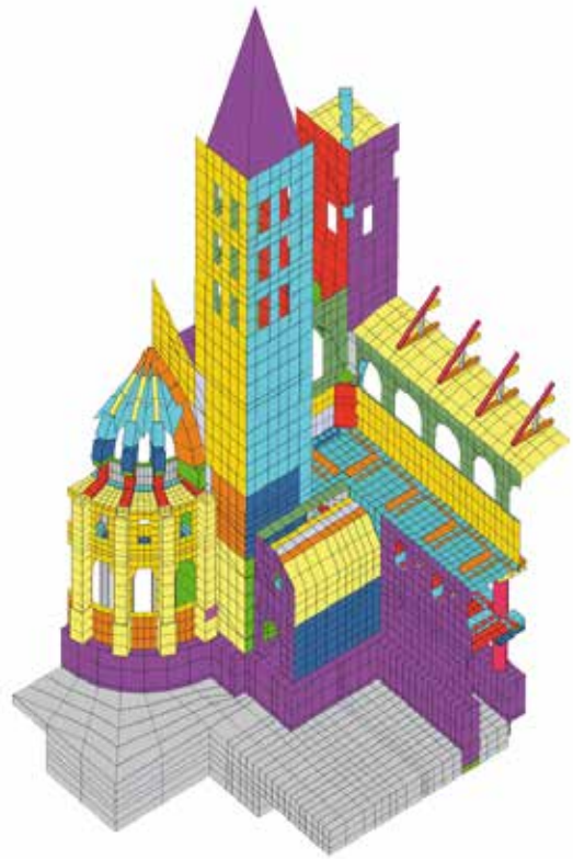
Model of the Brunin Tower including the soil heterogeneity
